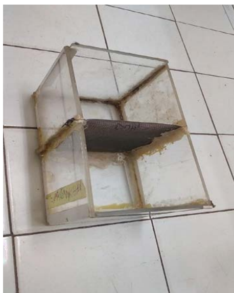
Figure 1. A) Electroreduction system B) Electrolysis cell with two compartments separated by a cationic membrane
