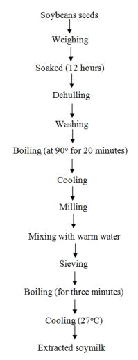
Figure 2. Flow diagram for extraction of Soymilk
