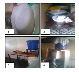
**Figure 7.** Filtration sieve after pasteurization (1), Pasteurization pan and pasteurized milk filtration fabric (2), Local manufacturing packaging machine (3), Foreign manufacturing packaging machine (4)
